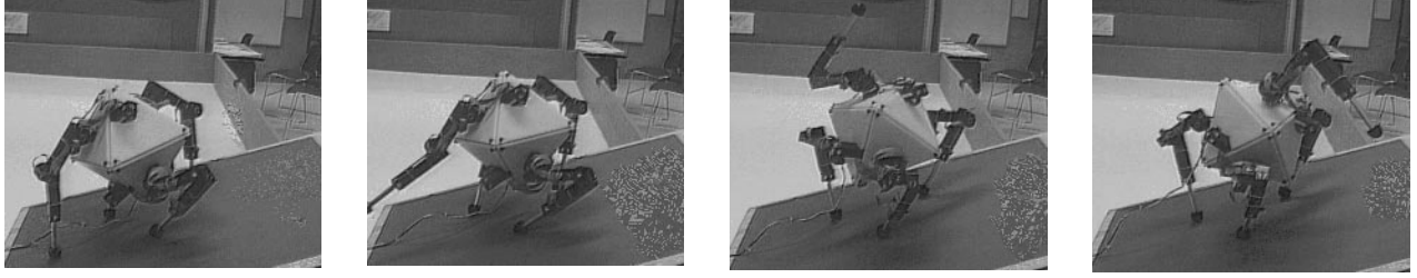
Figure 3: Canonical tumble with 4-beast prototype up a 20 degree slope (taken from [10]).
